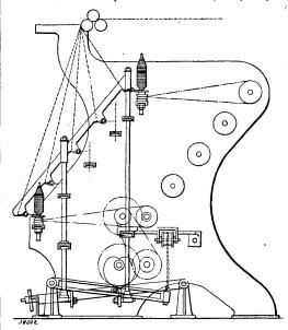
When the bobbin, tube, or quill is secured to the spindle, the drag is given entirely by the flyer, but if desired, it can be divided between the flyer and the bobbin, tube, or quill, by making a frictional contact between either of these and the spindle. (Accepted October 3, 1900.)
