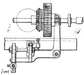
carriage, and the other arm of which is fitted with a fork located in a recess of the spurwheel which forms the roller box. The bell-crank lever is pivoted to the roller beam. It is stated that slipping of the roller box, breaking of wheels, cutting or damaging of the yarn through slipping out of gear, and wear and tear of the various parts are by this invention reduced to a minimum. (Accepted June 27, 1900.)
