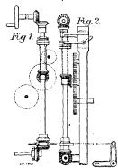
of gear by means of a hand lever. It will be seen that when the clutch is in gear, the shedding mechanism, "letting off" and "taking up" motions are all driven from the vertical shaft. When, however, the clutch is thrown out of gear, the long sleeve revolves loosely on the vertical shaft, and the latter can be turned back, the shedding mechanism, "letting off" and "taking up" mechanism, also being turned back at the same operation. (Accepted July 4, 1900.)
