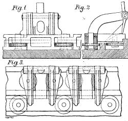
tion r ller being mounted between the fork, upon the pin that couples the forked end of the link to the tongue piece of the next link. Two studs carrying antifriction rollers are fixed in the underside of the clip. The peripheries of these rollers bear against the side of a rib on the guide rail, and the peripheries of the rollers carried by the forked end of the clip chain links bear against the side of a further rib on the guide rail. (Accepted June 2, 1900.)
