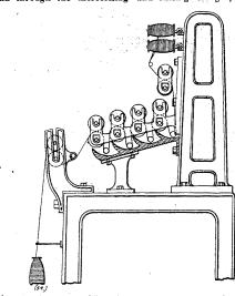
drying rollers, and on to bobbins on which it is wound when doubled and mercerised. The mercerising liquor and rinsing water may be circulated by means of pumps connected with storage cisterns. (Accepted February 21, 1900.)
