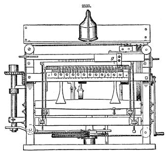
formed in the needle-cylinder, they are forced up and down as desired. Each row of loops is also sustained until the next is formed by means of the needles themselves, as the needle-cylinder prevents their bending inward, and keeps them in a vertical position. The cam-cylinder is moved by a bevel-gear connected to a driving-crank, and when moved continuously in one direction knits a circular web, which may be narrowed as desired by removing needles and placing their loops on adjacent needles.
