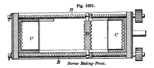
press-boxes C C alternately, and is operated by four screws B B simultaneously driven, one at each corner, two showing in the illustration, which is a side elevation.
