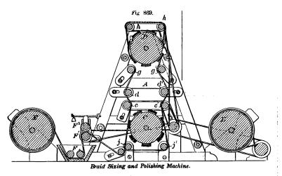
from a toothed wheel actuated by projections on the end of the lower brush-shaft engaging with the teeth.
