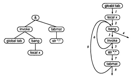
Each node of the parse tree is attributed by the edges set of the corresponding sub-expression. For example, the edges set for local x contains edge 2, the set for bang contains edges 2-4, the set for invoke contains 1-6, etc.
