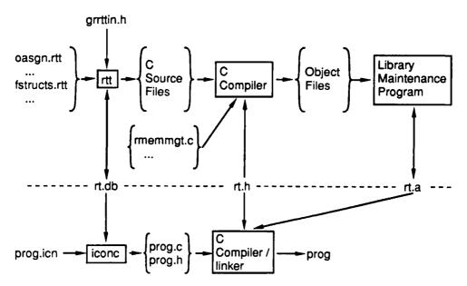
rtt automatically invokes the C compiler and the library maintenance program. The person adding run-time operations to the compiler has a simplified view of the run-time system:
